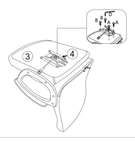
STEP 5: Place mechanism 4 on gas lift 5.
